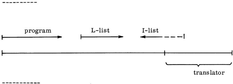
The I-list starts at the high end of the store and has an extension reading into the translator for the fixed (pre-declared) identifier such as `sin`, `read`, etc.
