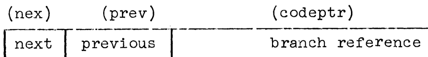
Figure 16. Data fields of auxiliary transfer list item. (Names in parentheses give field reference modes used in Tables II, III, and IV.)
