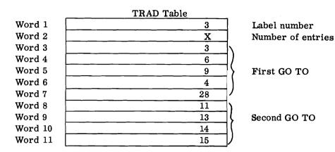
The TRAD record is generated during the processing in Section 1. It is entered on tape 2, file 5, as record 7 in Fortran II and 709 and record 3 in Fortran I. The first word of the first record is the label number three. The second word of the first record is a binary count of the number of words in the TRAD record.
