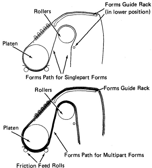
The diagrams at the left show the proper forms path for singlepart and multipart forms. The steps to insert forms begin below.
