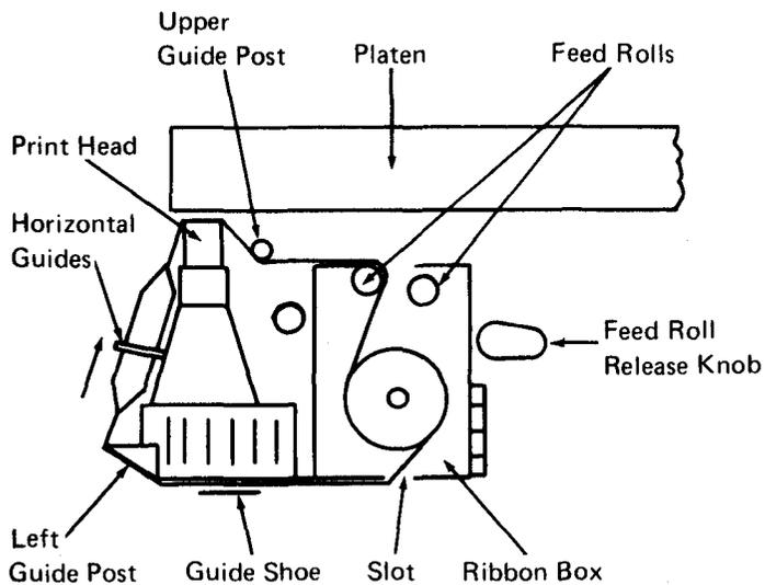
14. Thread the part of the loop nearest the platen between the feed rolls and on the inside of the upper guide post.
