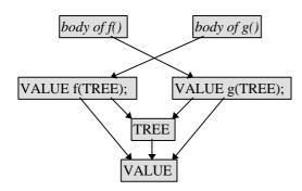
This structure has the advantage that any valid program would be represented by an acyclic directed graph (at least after the initial compilations during which dependencies are generated).
