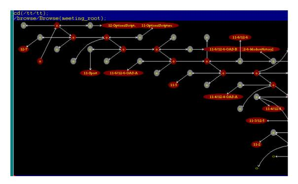
This display shows a real-life data-structure as used by a program called 'tt'. 'tt' is discussed in Chapter 11. This data-structure is a linked list with associated objects, and can be seen extending from left to right across the above diagram.
