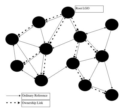
The above diagram shows the two types of references: 'ordinary references', i.e. an LGO pointer, as an ordinary value in Barbados's type system, and 'ownership links'.
