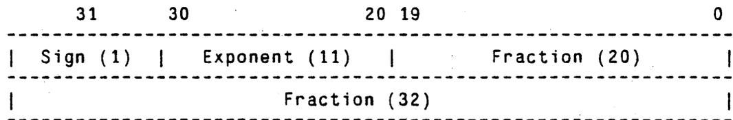
The exponent is biased by 1023. Exponents of 0 and 2047 are reserved. The most significant bit of the fraction is stripped off since it is always the complement of the sign bit, and carries no information.
