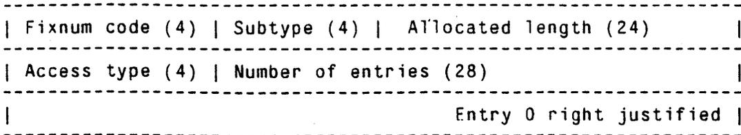
Note that the subtype field overlaps the type field -- this means that the subtype can change the sign bit of the fixnum. The first word of an I-Vector contains the Fixnum type-code in the top 4 bits, a 4-bit subtype code in the next four bits, and the total allocated length of the vector (in 32-bit words) in the low-order 24 bits. At present, the following subtype codes are defined:
