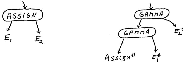
Figure 4.2-8: Standardization of Simultaneous Assignment
