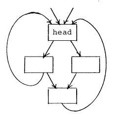
The interval forms a programming locality which may contain variable names not defined or used elsewhere in the program. The compacted use-definition chaining algorithm attempts to take advantage of this hypothesis by restricting usedefinition chains to these localities. Putting it another way, a variable used inside an interval may have been defined in one of two ways:
